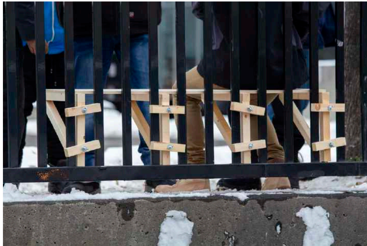
Fig. 39: The temporary installment method I designed to hang the bench.
