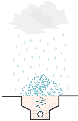
Bioswales collecting and filtering rain water
